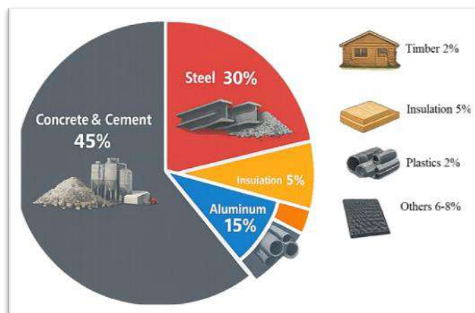
Figure 2. Representative proportional contribution of primary construction materials to embodied carbon in building assemblies.
